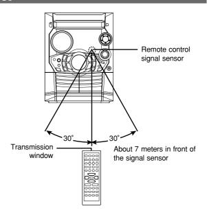
Aim at the sensor, avoiding obstacles, at a maximum range of 7 meters directly in front of the unit.
